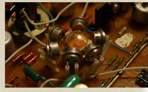
Here is a picture of the photo-optical heart of the Estradin Phaser, notice the six photocells surrounding the little light bulb.
